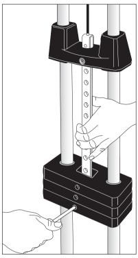
Hold the stem in place by inserting the Weight Pin (through a weight) near the base of the Selector Stem.
